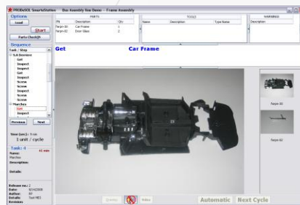
Automatic Work Instruction Generation
